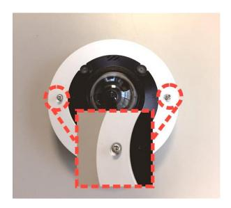
Place the camera at the installation location. Mark the position of the two screw holes indicated in the right figure on the ceiling or wall. Then draw a line along the concave edge of the camera to indicate the cable position.
