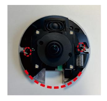
3. On the ceiling or wall, draw a dot 20 mm above the center of the marked concave edge. Set the marked dot as the center, and draw a cable entry hole with 30 mm diameter (radius 15 mm).
