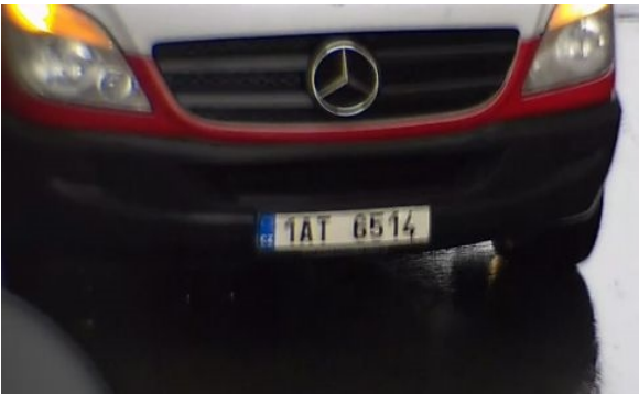
Fig. 15: Blurred license plate due to long exposure time
