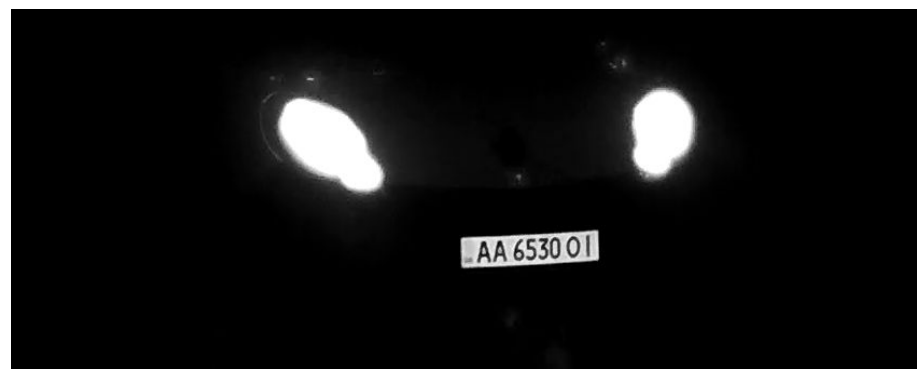
Fig. 11: Easily readable license plate at night with infrared LED illumination
