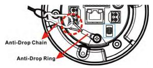
NOTE: For safety concern, it is recommended to hook up the camera with the anti-drop chain of the pendant when installing the camera. For more information about pendant and anti-drop chain, please contact the camera manufacturer.
