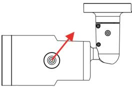
3. The positions of microSD card slot and default button are as shown.
