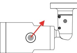
3. The positions of microSD card slot and default button are as shown.
