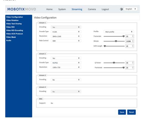
In the **Streaming** submenu, the administrator can configure specific video resolution, video compression mode, video protocol, audio transmission mode, etc. Further details of these settings will be specified in the following sections.
