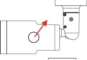
2. Open up the internal cover using a security torx.
