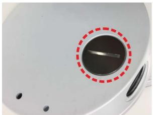
Place the camera at the installation location. Mark the position of the two screw holes and the back conduit entry (for cable entry use) indicated in the right figure on the ceiling or wall.
