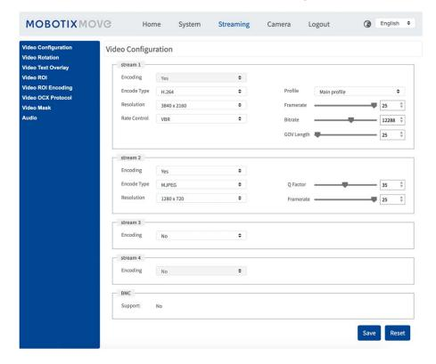
In the **Streaming** submenu, the administrator can configure specific video resolution, video compression mode, video protocol, audio transmission mode, etc. Further details of these settings will be specified in the following sections.
