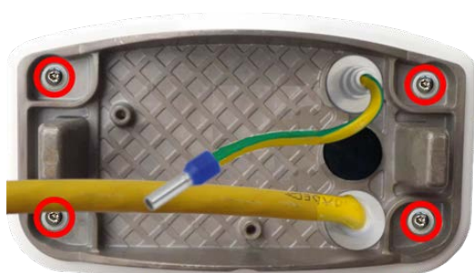
Fig. 54: Mounting plate with ground wire and network cable
