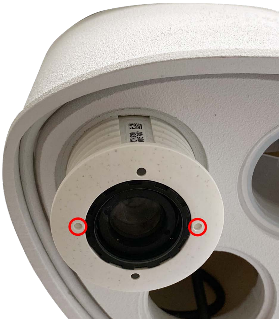
Fig. 22: Unlock the sensor module
