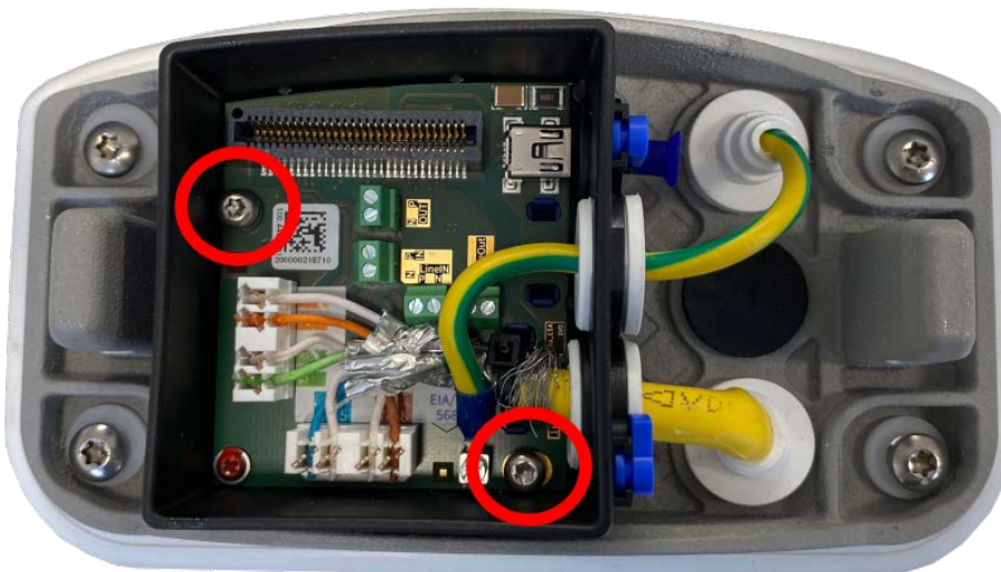
Fig. 63: Mount the Connector Box LSA (top view) using the two screws (highlighted red in the figure) on the mounting plate
