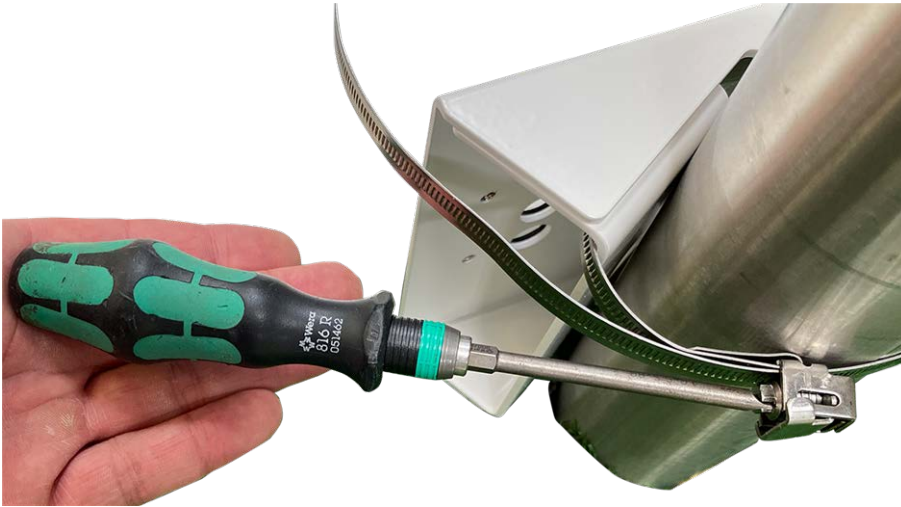
Fig. 42: Tighten the straps
