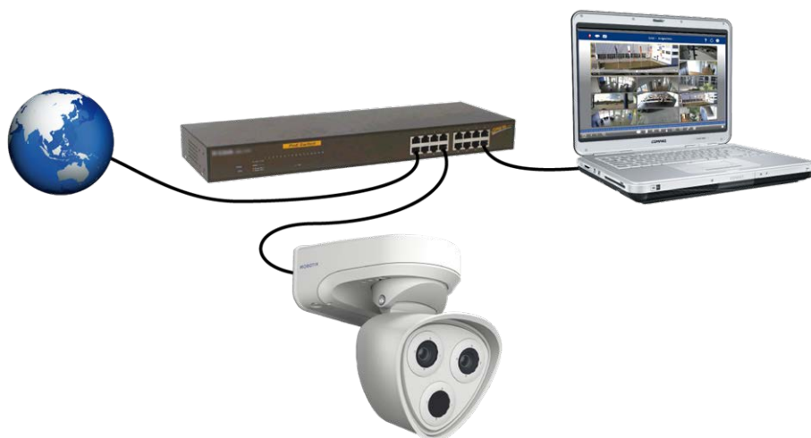
Fig. 51: Power supply using PoE switch according to PoE Plus (802.3at-2009).
