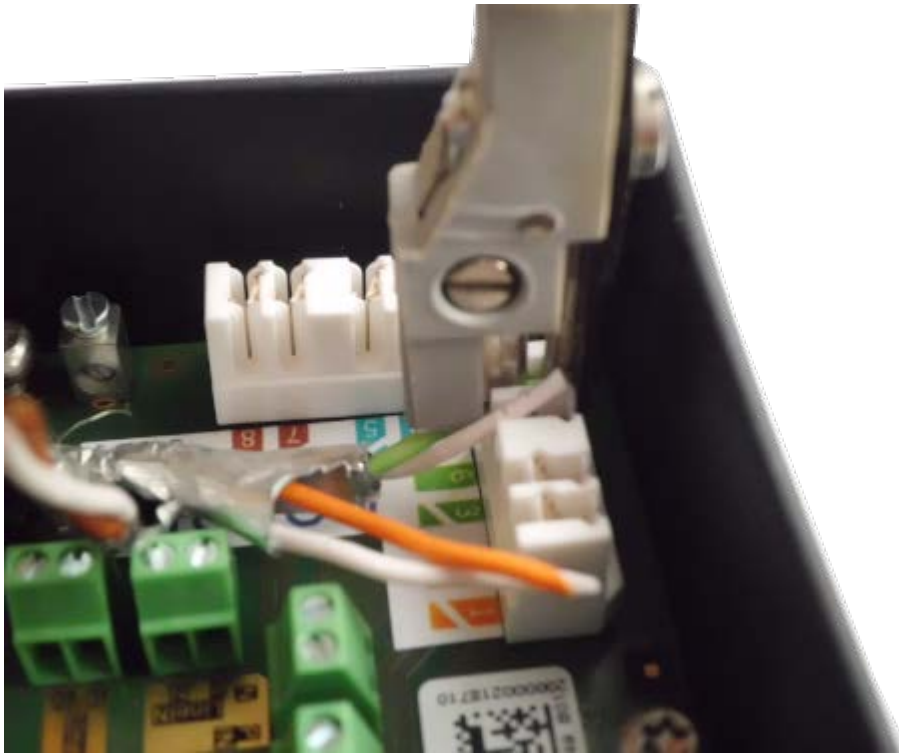
Fig. 59: Network wires connected using LSA+/Krone tool
