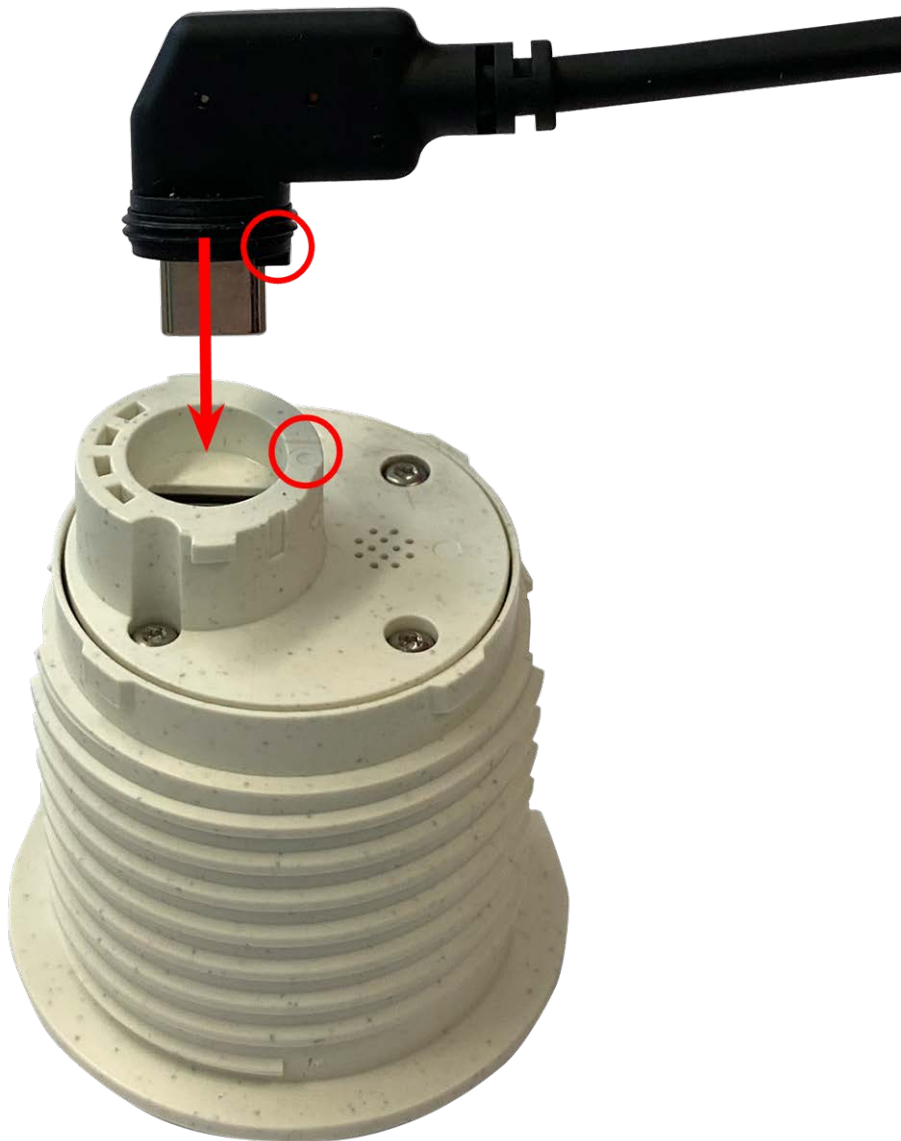
Fig. 9: Connect the sensor module cable
