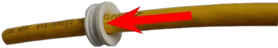
Fig. 55: Network cable with rubber plug C.5
