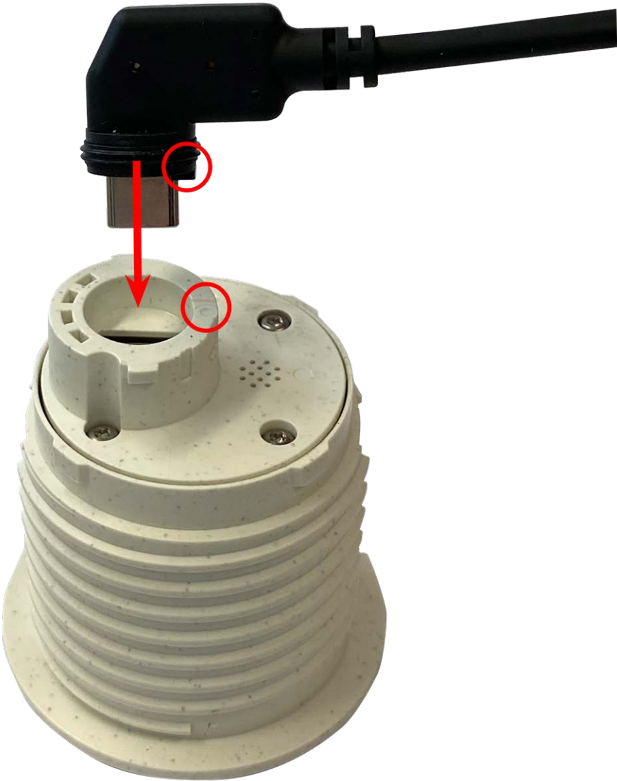
Fig. 27: Connect the sensor module cable
