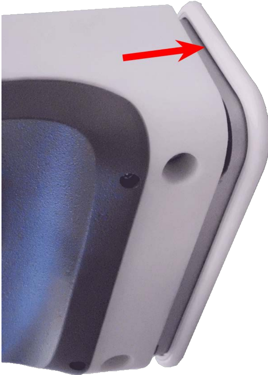
Fig. 68: Press camera onto mounting plate
