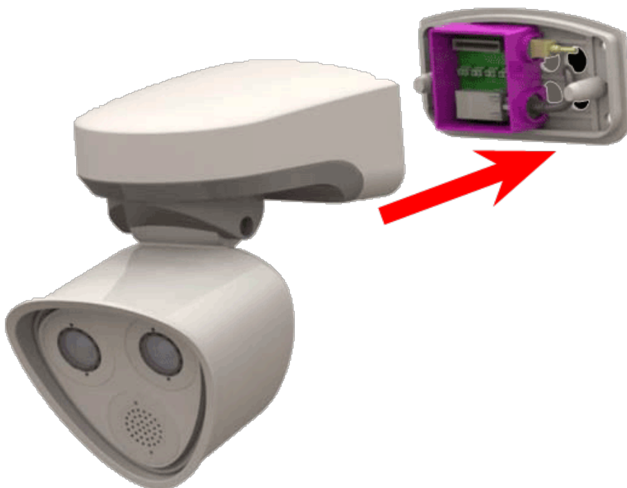
Fig. 67: Attach the camera on the mounting plate to complete the mounting of the camera
