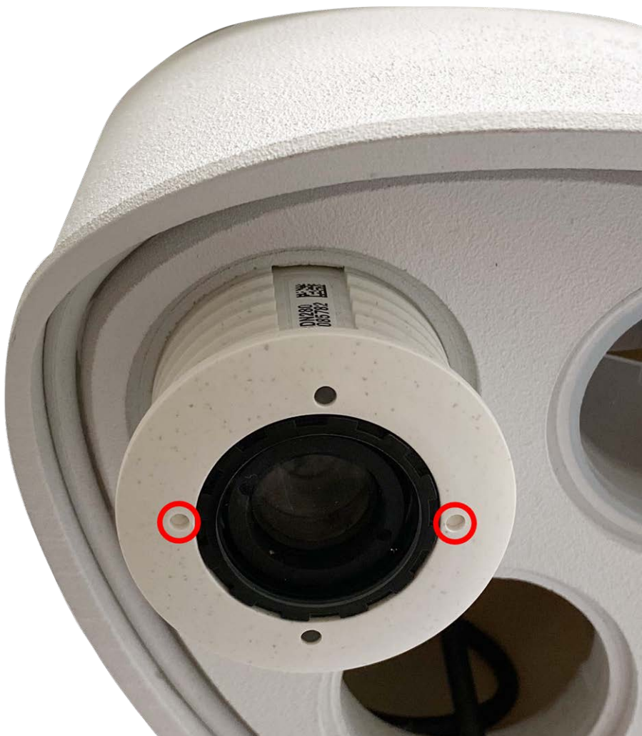
Fig. 12: Insert sensor module into module housing
