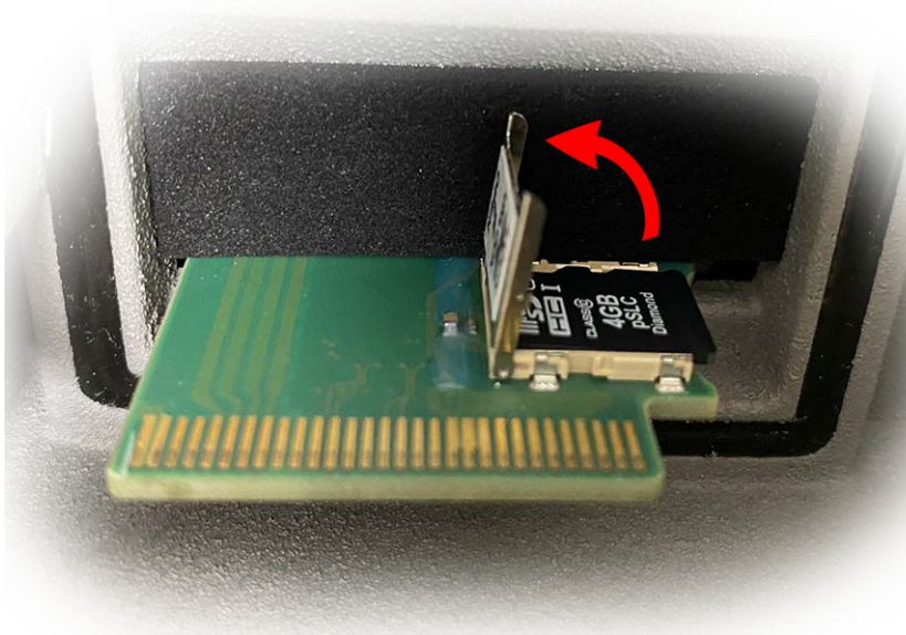
Fig. 93: Unlock microSD card holder
