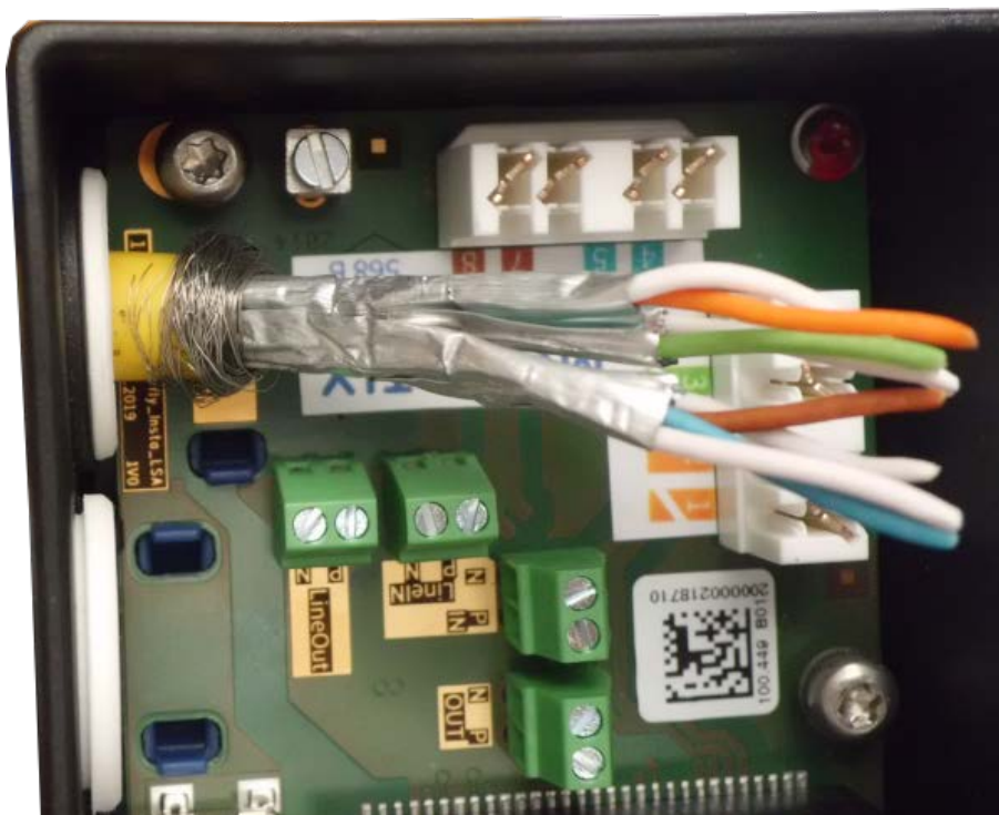
Fig. 56: Network cable inserted, plug properly seated
