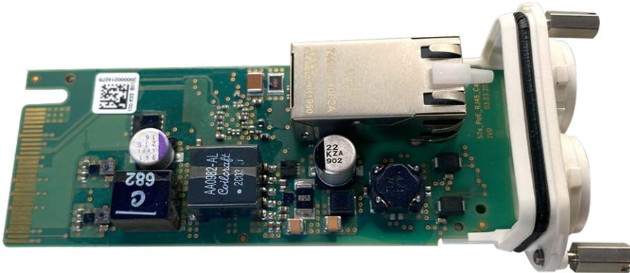
Abb. 17: S74 Network slide in board with RJ45 socket
