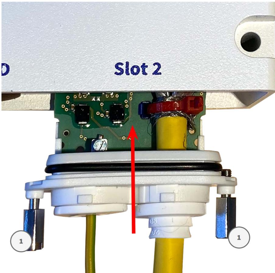
Abb. 30: S74 network slide in board with LSA terminal anschließen
