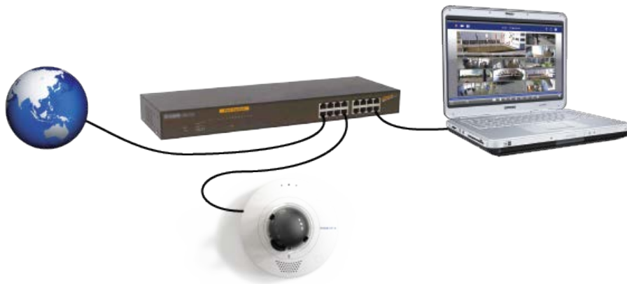
Fig. 15: Power supply using PoE switch according to PoE Plus (802.3at-2009).
