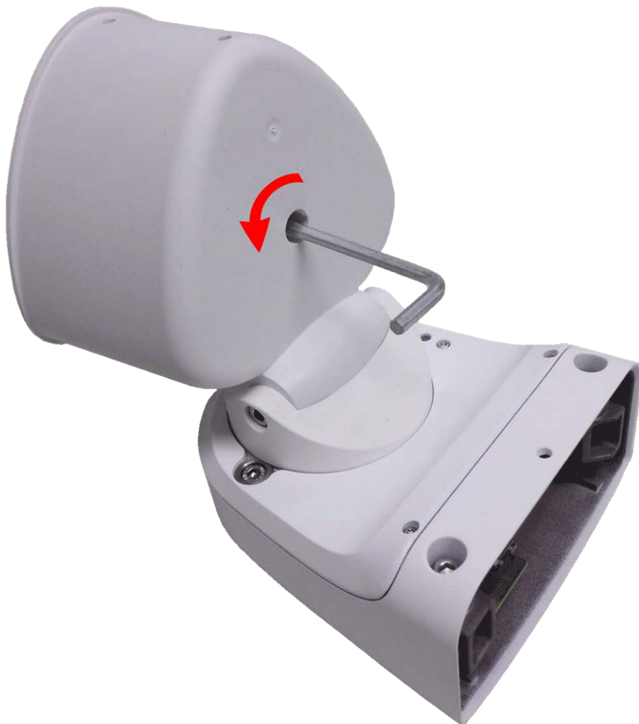
Fig. 14: Opening the module housing
