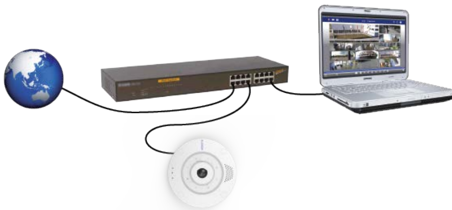
Fig. 15: Power supply using PoE switch according to PoE Plus (802.3at-2009).
