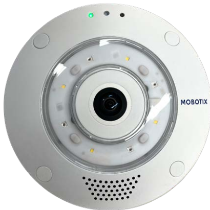
Fig. 17: Camera LED on top of the camera body
