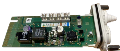
Fig. 20: S74 Network slide in board with LSA terminal
