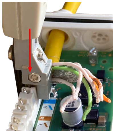
Fig. 26: Network wires connected using LSA+/Krone tool
