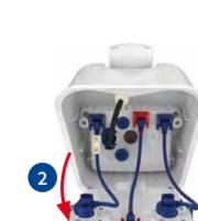
Using the Allen wrench, **cautiously** push from behind **in an alternating fashion** onto the left and the right bolt **1** and push the front element out of the front of the housing.
