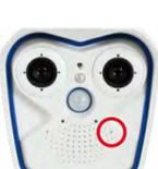
The LED now flashes once and repeats the flash signal after pausing for one second (the number of flashes indicates the current boot option). To go to the next boot option, briefly press the key again (< 1 sec). After the last boot option, the camera returns to the first option (LED flashes once).
