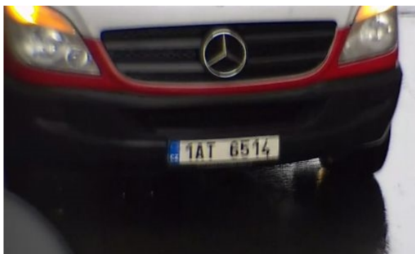
Fig. 13: Blurred license plate due to long exposure time
