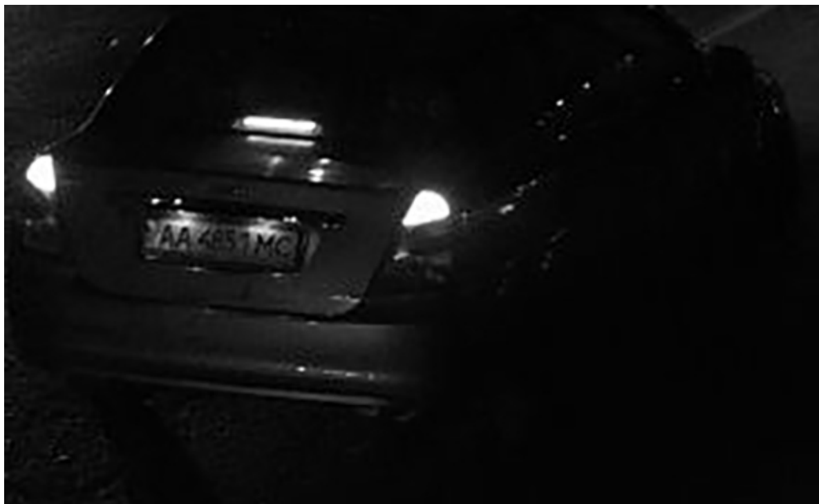
Fig. 16: Insufficient light to recognize license plate
