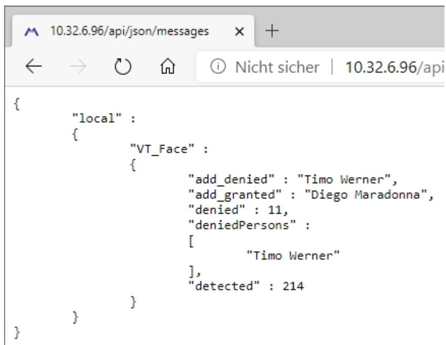
Fig. 19: Example: Meta data transmitted within an MxMessage of the Visage Technologies Face Recognition App
