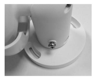
If the screw holes are blocked by the camera body, loosen the screw shown in the right figure but do not detach it. Then rotate the camera body to reach the screw holes.
