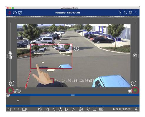
Fig. 78: Adding Clips for Exporting in the Playback View
