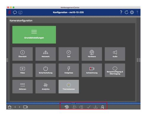
Fig. 163: Applying and saving changed settings
