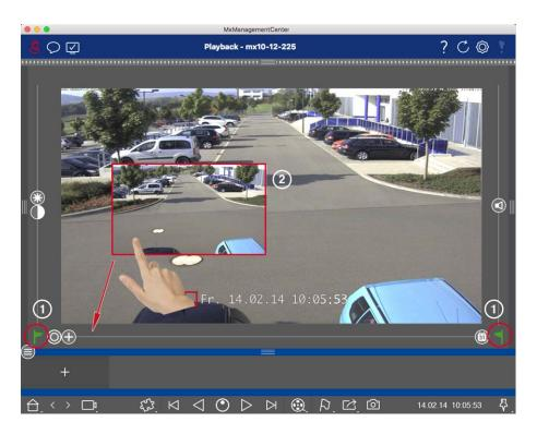
Fig. 11: Adding Clips for Exporting in the Playback View
