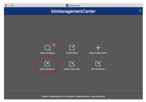
Fig. 52: Importing configurations from MxControlCenter
