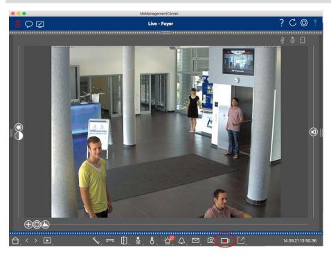
Fig. 6: Manually recording live images
