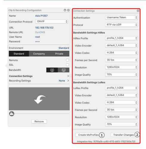
Fig. 116: Connection Settings (MOBOTIX MOVE/ONVIF Cameras)
