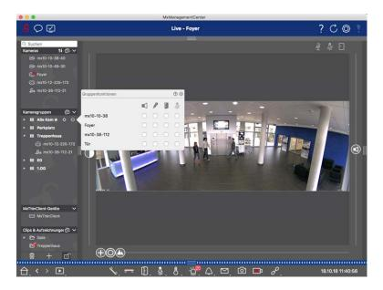
Fig. 100: Assigning group functions
