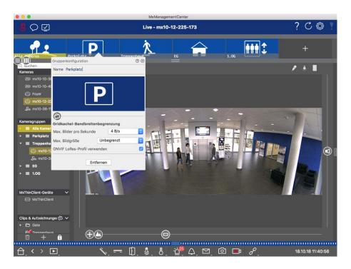
Fig. 101: Limiting the frame rate of live images
