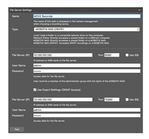
Fig. 145: MOBOTIX NAS settings
