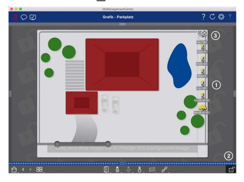
Fig. 96: Changing the camera position on the background image
