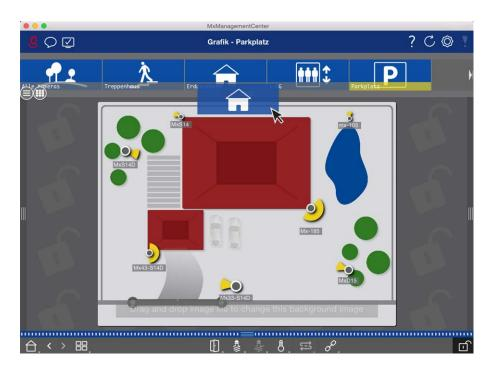
Fig. 98: Dragging additional camera group onto the background image
