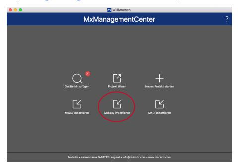
Fig. 53: Importing Configurations From MxEasy
