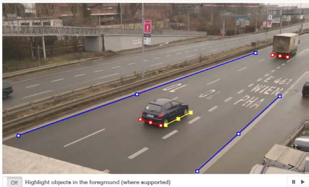
Fig. 94: Draw a reference line (yellow) and give a reference length
