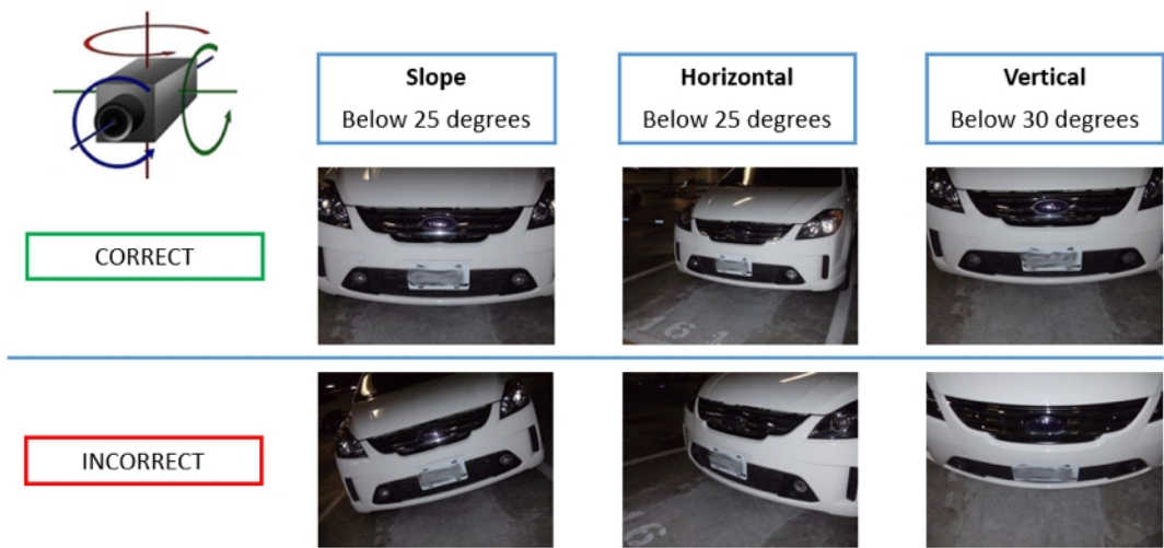
Fig. 11: Maximum rotation angle
