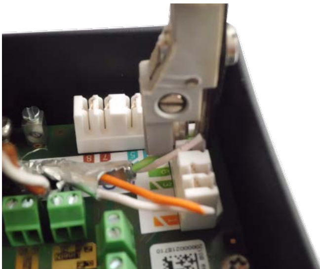
Fig. 59: Network wires connected using LSA+/Krone tool
