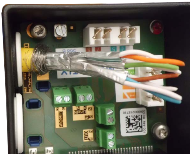
Fig. 56: Network cable inserted, plug properly seated
