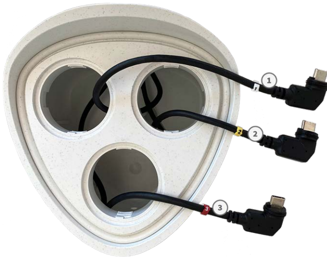
Fig. 8: Numbered sensor module cables
