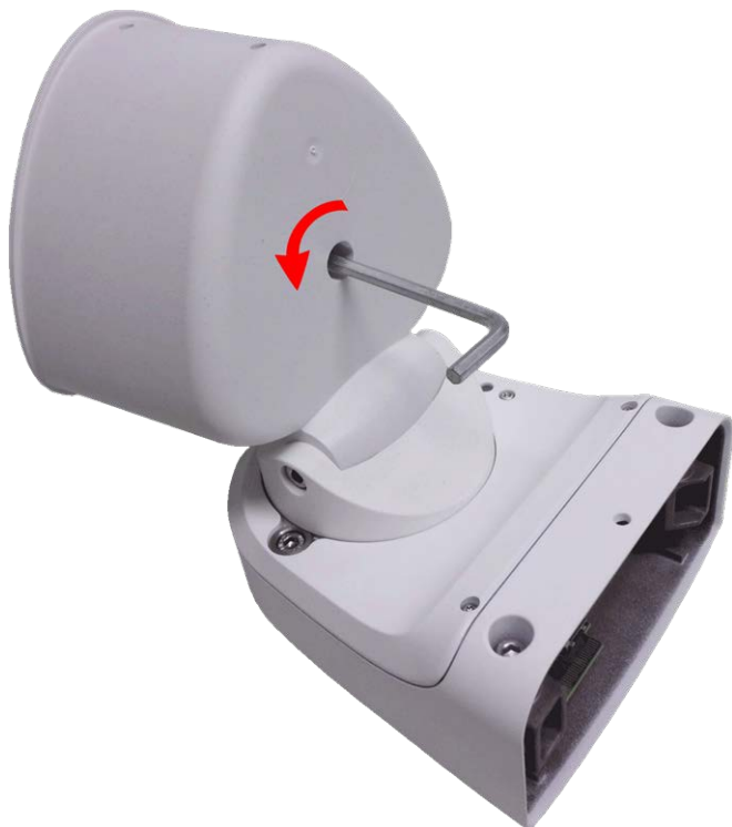
Fig. 14: Opening the module housing
