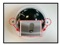
**Step 2:** The dome cover is attached to the camera housing with an anti-drop cable. Loosen the screw indicated in the right figure to detach the dome cover from the camera housing.
