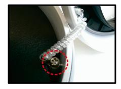
**Step 3:** Choose a suitable conduit entry on the camera for cable connection (side conduit entry or back conduit entry). If users are using the back conduit entry for cable connection, please use a coin to open the conduit entry block and place it to the side conduit entry.
