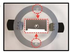
**Step 10:** Put the camera into the ceiling opening, and fix the U-shaped Bracket on the T-bar Bracket by tightening the two screws shown in the figure.
