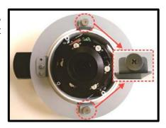
**Step 11:** Put the Ethernet cable through the chosen conduit entry hole, and connect it to the camera.
