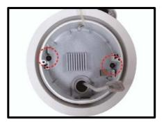
**Step 13:** Place the camera module back to the camera housing. Align the two screw holes of the camera and fasten the two screws.
