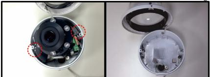
**Step 12:** Put the camera housing to the pendant cap and fasten the camera housing to the pendant cap with the supplied M4x8 mechanical screws.
