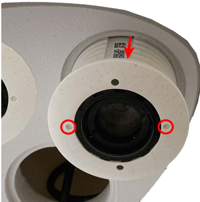
Fig. 23: Remove sensor module from the module housing
