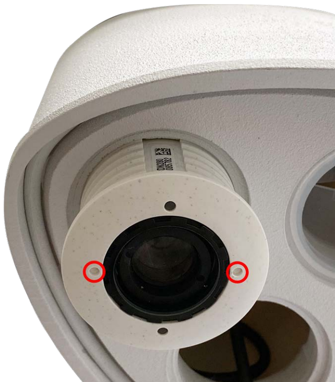
Fig. 12: Insert sensor module into module housing
