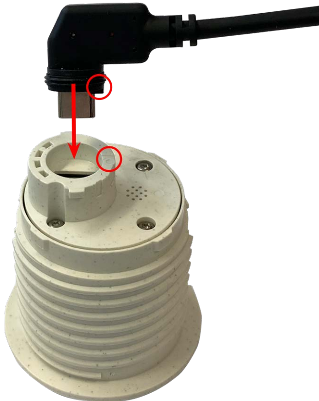
Fig. 9: Connect the sensor module cable
