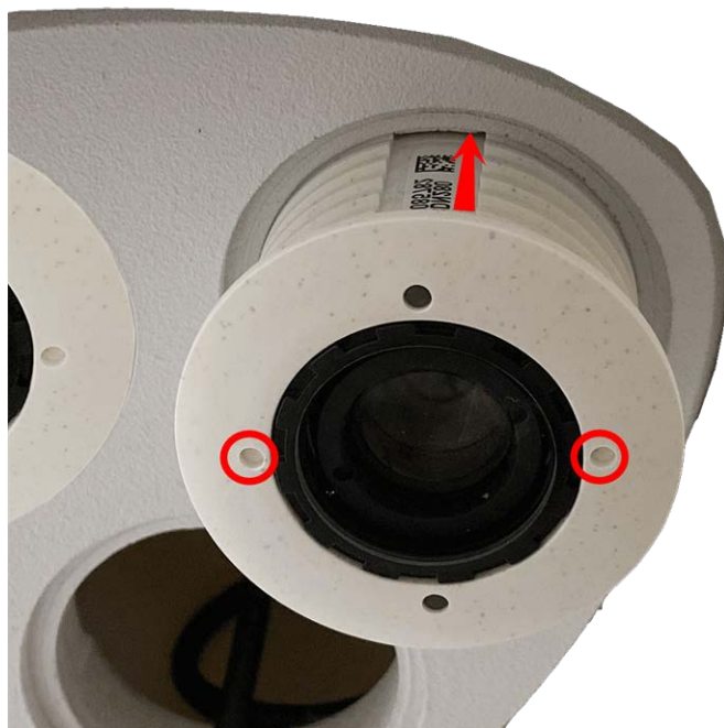
Fig. 25: Insert sensor module into Thermal front plate
