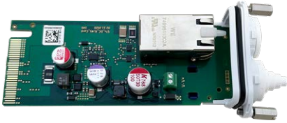
Fig. 30: S74 Network Slide in Board with RJ45 and VDC power supply
