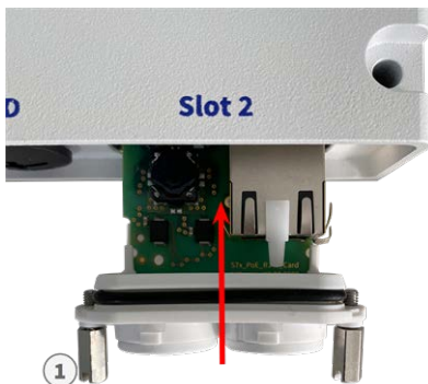
Fig. 19: Connecting the S74 Network Slide in Board with RJ45 socket
