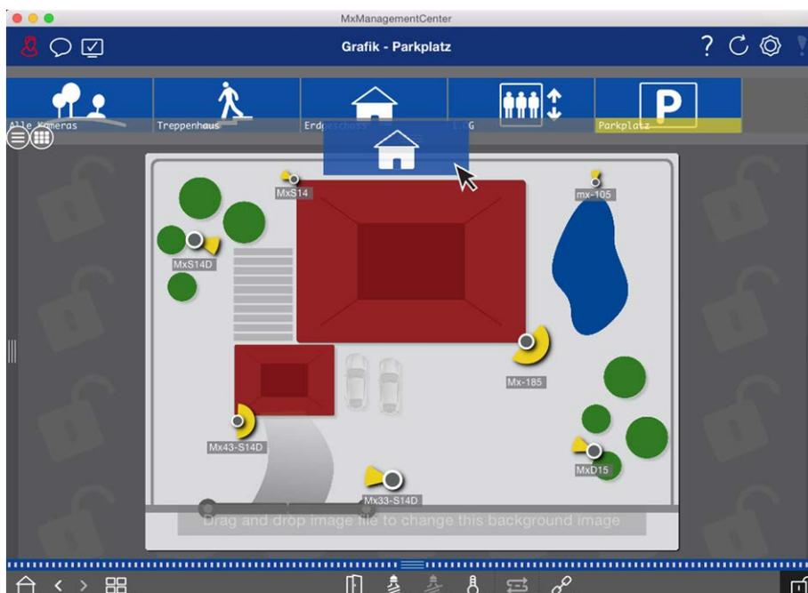
Fig. 94: Dragging additional camera group onto the background image
