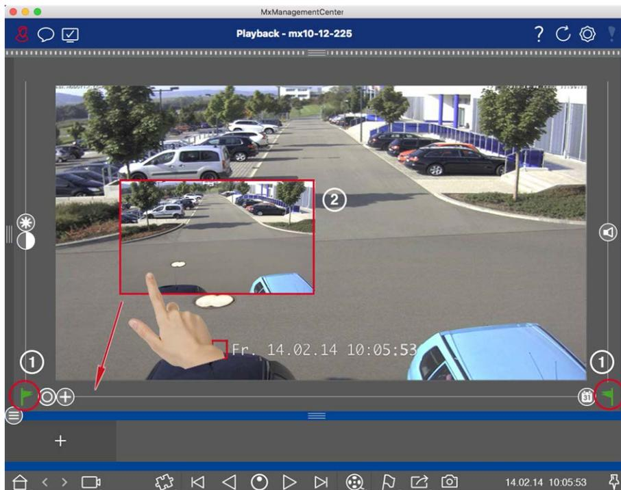
**Fig. 88: Adding Clips for Exporting in the Playback View**
