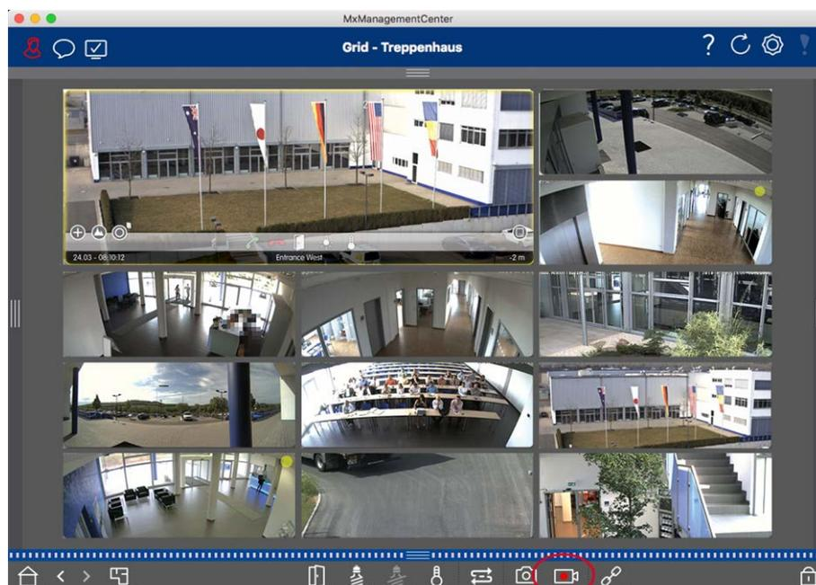
Fig. 63: Manually recording live images
