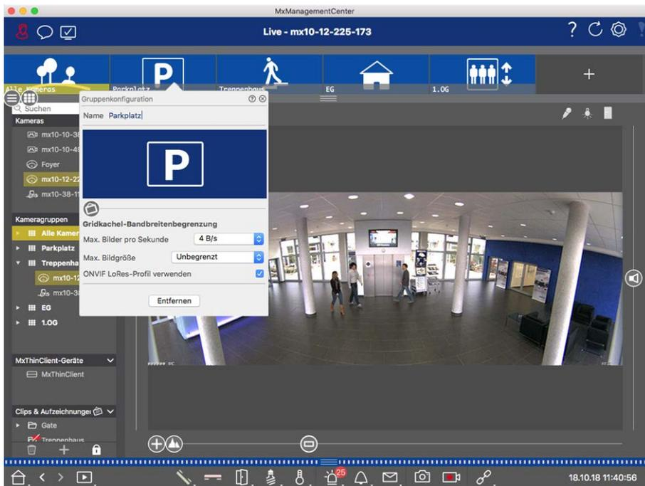
Fig. 97: Limiting the frame rate of live images
