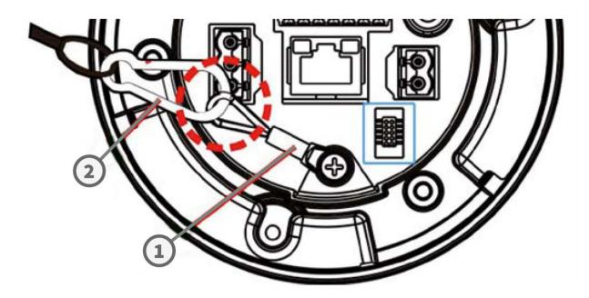
**NOTE!** For safety reasons, it is recommended to hook up the camera's anti-drop ring ① with the anti-drop chain ② of the pendant when installing the camera. For more information about the pendant and anti-drop chain, please see the corresponding Quick Installation document available at **www.mobotix.com** > **Support** > **Download Center** > **Marketing & Documentation** > **Manuals** in the **Speed Dome Accessories** section..
