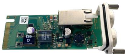
Fig. 17: S74 Network Slide in Board with RJ45 socket
