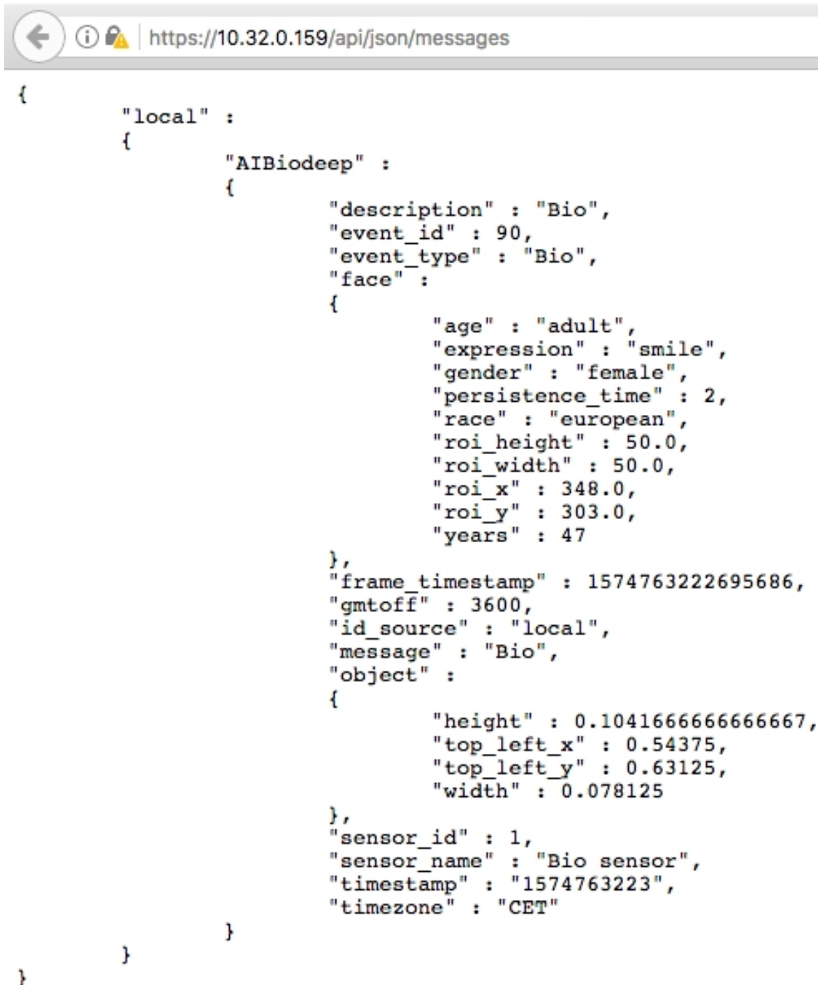
Fig. 15: Example: Meta data transmitted within an MxMessage of the AI-BIO app
