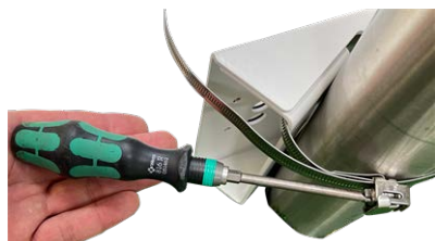
Fig. 14: Tighten the straps
