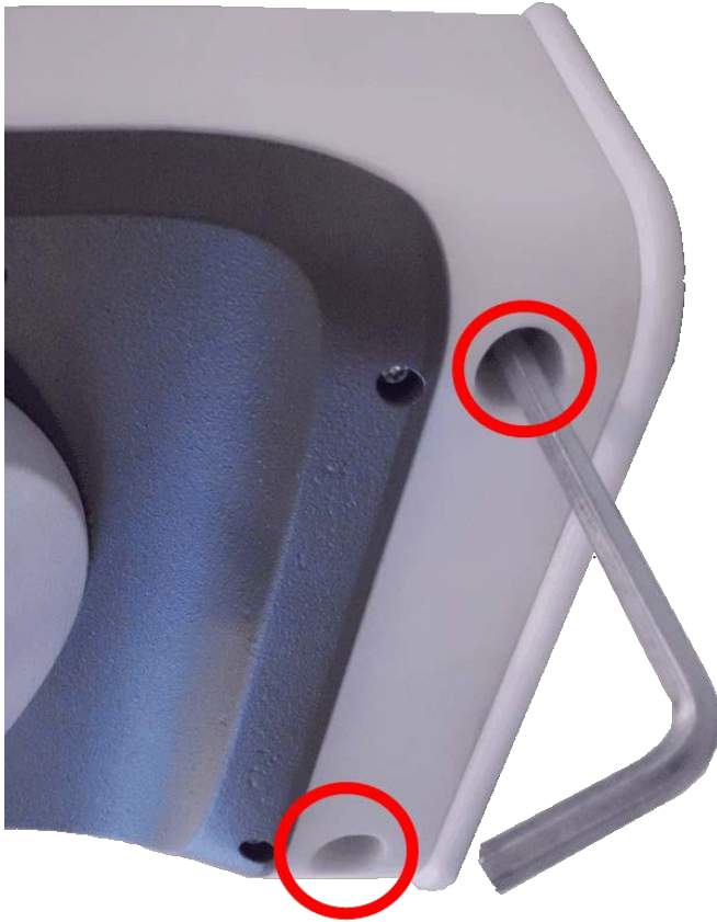
Fig. 71: Tighten Allen screws
