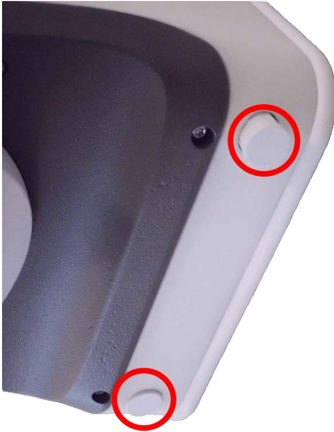
Fig. 92: Remove rubber plugs
