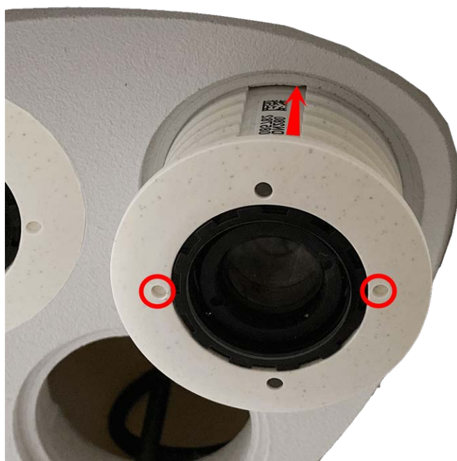
Fig. 26: Insert sensor module into Thermal front plate
