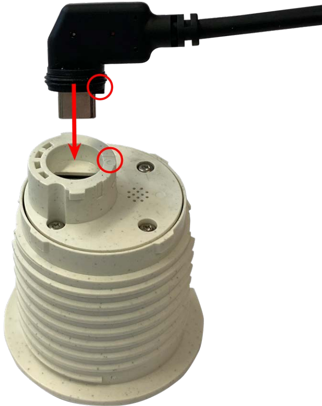
Fig. 28: Connect the sensor module cable
