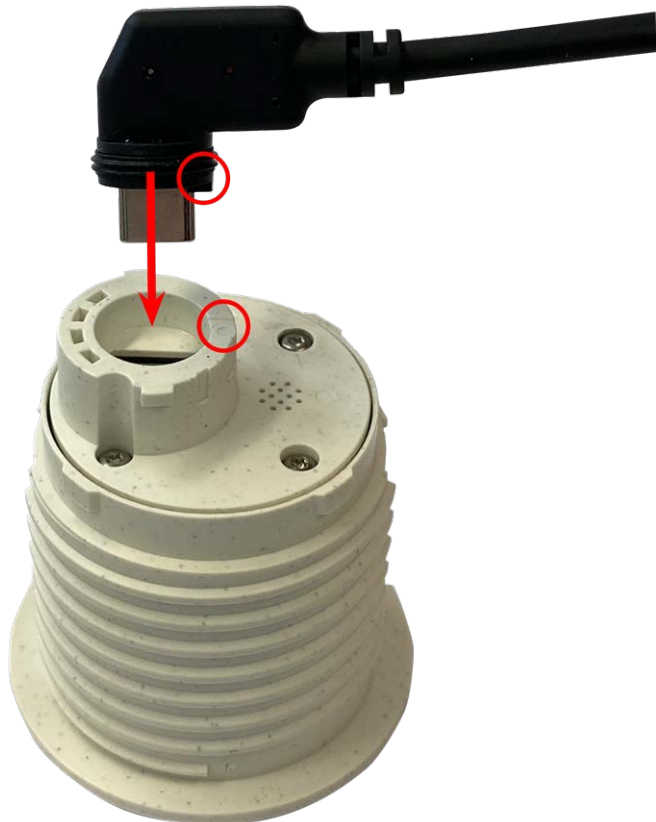
Fig. 10: Connect the sensor module cable
