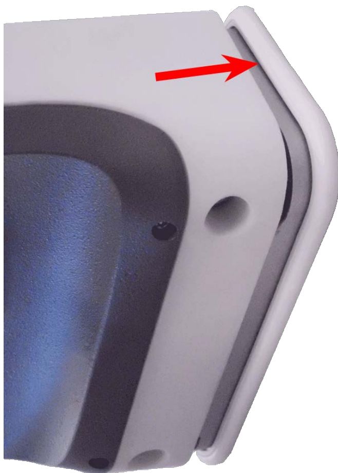
Fig. 70: Press camera onto mounting plate
