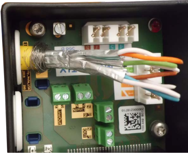
Fig. 57: Network cable inserted, plug properly seated
