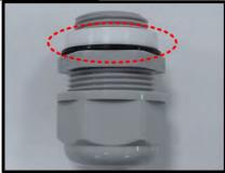
**Step 8:** Loosen the thread-lock sealing nut of the cable gland. Then thread the Ethernet cable through the sealing nut and the gland body. If there are other cables, such as power cable, alarm I/O cable or audio I/O cable, please also insert them through the sealing nut and the gland body.
