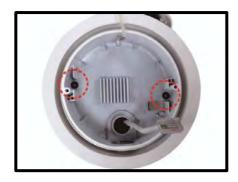
**Step 13:** Place the camera module back to the camera housing. Align the two screw holes of the camera and fasten the two screws.
