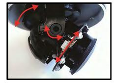
**Step 16:** Attach the dome cover to the camera, align the arrow mark on the dome cover with the one on the camera housing and fasten the two security screws. And the pendant cap mount installation is completed.
