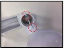
**Step 6:** Insert the spring washer-8 followed by the pendant tube washer and the rubber washer-8 to the supplied M8x16 hex head stainless steel screw. Then fasten the screw.
