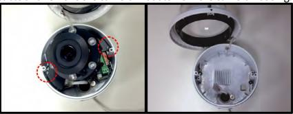
**Step 12:** Put the camera housing to the pendant cap and fasten the camera housing to the pendant cap with the supplied M4x8 mechanical screws.
