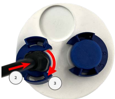
Fig. 16: Press the plug in firmly until the blue sealing ring clicks into place
