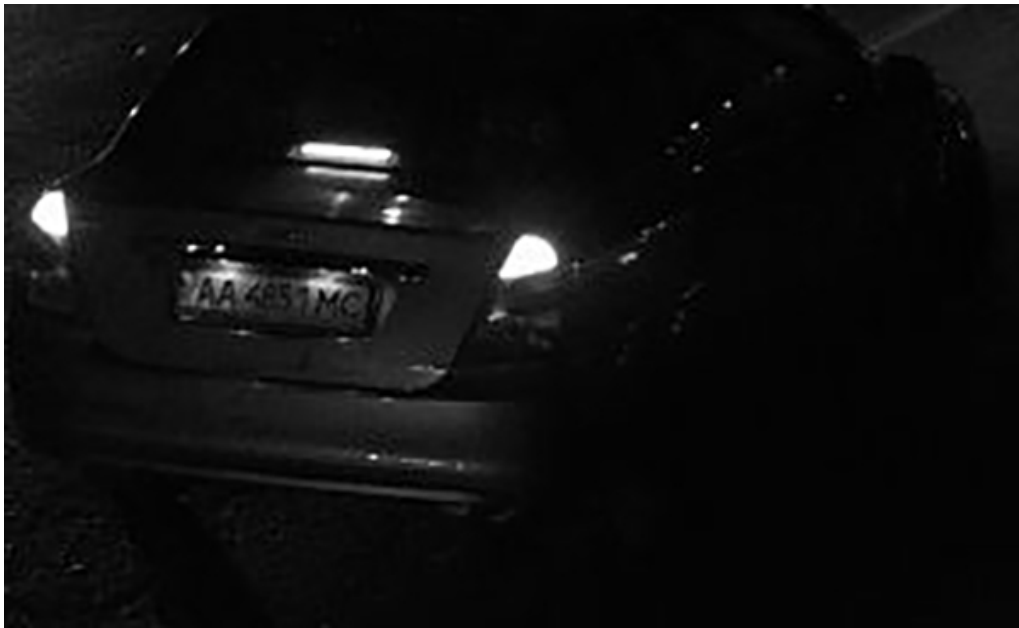
Fig. 16: Insufficient light to recognize license plate
