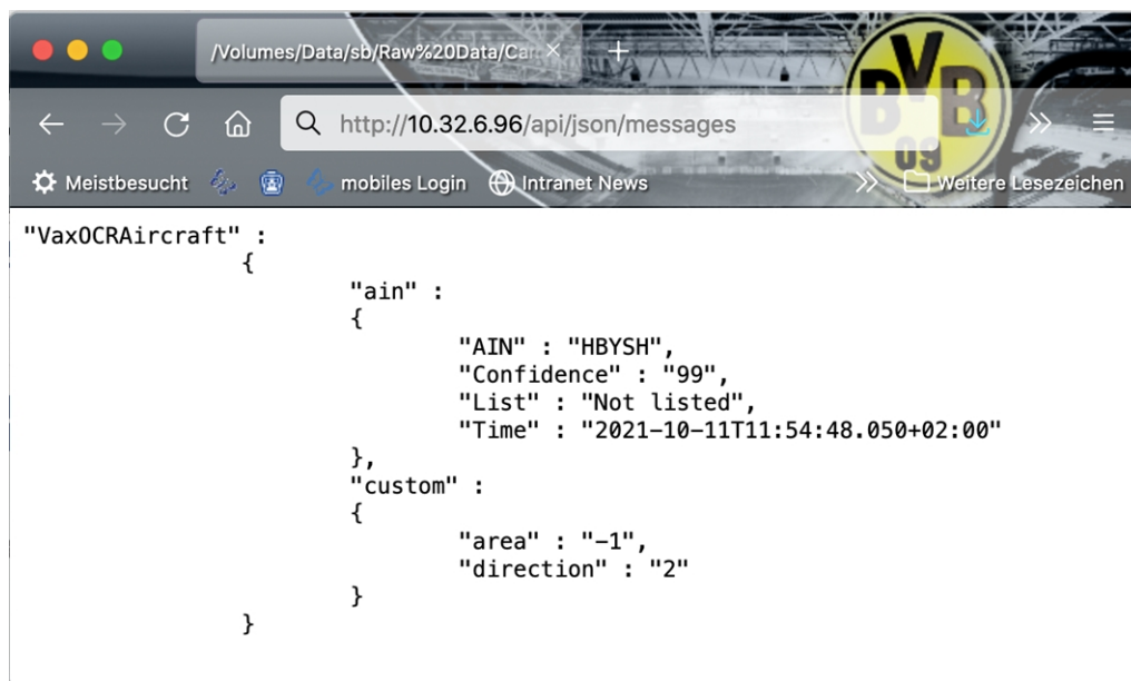
Fig. 30: Example: Meta data transmitted within a MxMessage of the Vaxtor Aircraft Identification Number Recognition App
