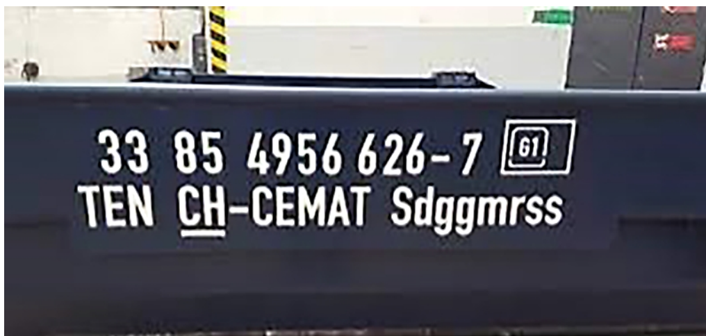
Fig. 26: UIC code on a railroad wagon
