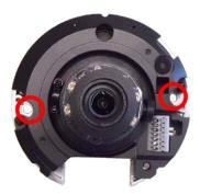
7. Attach the dome cover to the camera and fasten the two Phillips screws.
