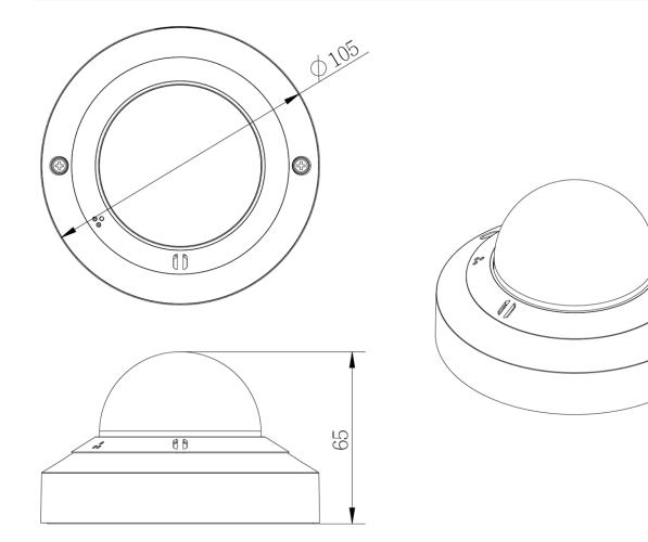
Fig. 1: 5MP Indoor Micro Dome Camera: All measurements in mm
