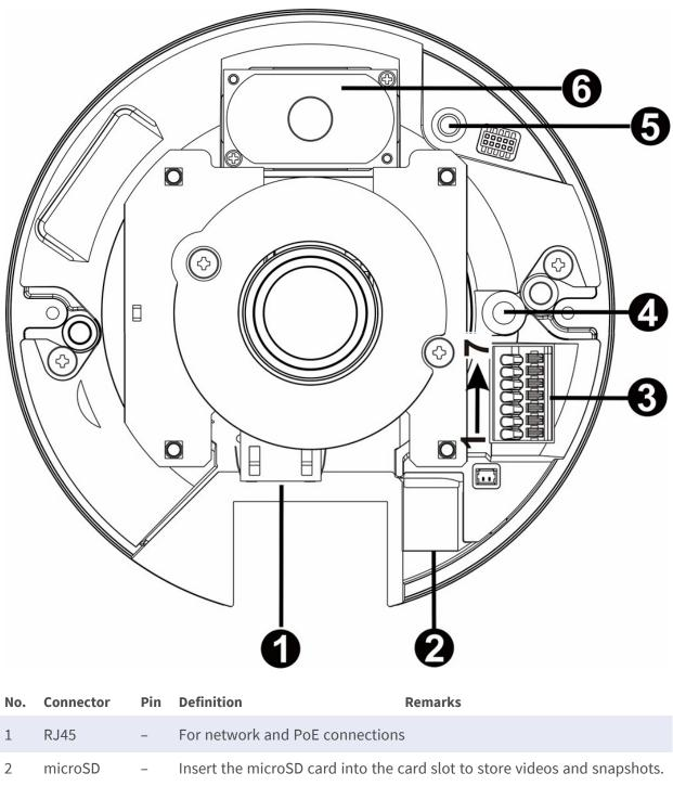
Card Slot Do not remove the microSD card when the camera is powered on.
