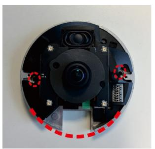
On the ceiling or wall, draw a dot 20 mm above the center of the marked concave edge. Set the marked dot as the center, and draw a cable entry hole with 30 mm diameter (radius 15 mm).
