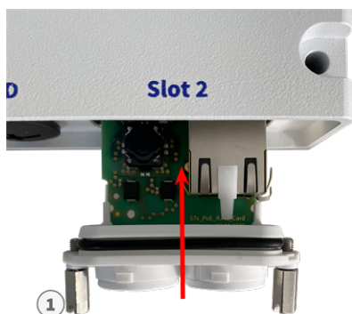
Abb. 19: S74 Network Slide in Board with RJ45 socket anschließen
