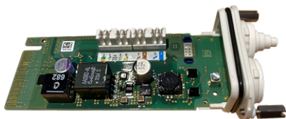
Abb. 20: S74 Network Slide in Board with LSA terminal
