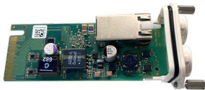
Abb. 17: S74 Network Slide in Board with RJ45 socket
