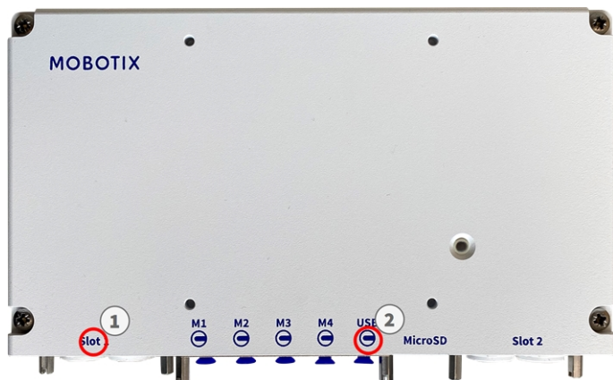
Fig. 3: CNPP compliant connection to the S74 Camera
