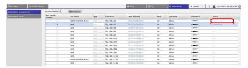
After the setting, there would be three possible situations. One is successfully **monitoring**. The other situation is **backup status activated**. The **offload** situation only happens after the primary NVR failure is fixed.
