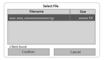
3. Select the preferred firmware (\*.zip/txz/txz.sha512) file and click **Confirm** to start the firmware upgrade progress. The NVR will automatically reboot after the system finish firmware upgrade.
