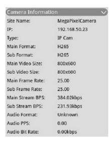
You can check brief summary of the selected IP camera. Click on any IP camera channel from the View Management's Camera View list or from the display layout to see the basic information. Camera information should include site name, IP address, device type, video format, etc.
