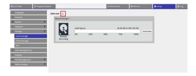
**NOTE!** If HDD is removed during operation (hot-swappable), please click the refresh icon next to **Disk List** to display current workable HDDs.
