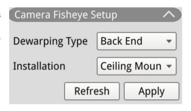
icon will appear on the bottom-right corner of the channel grid. includes **Normal View**, **PTZ View**, **360 View**, **Quad View**, **OPR View**, and **103R View**. Select preferred mode and the NVR will automatically dewarp the source images from fisheye.
