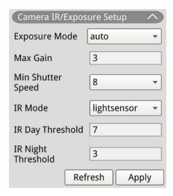
The NVR allows users to configure the IR function and exposure settings of the IP camera.
