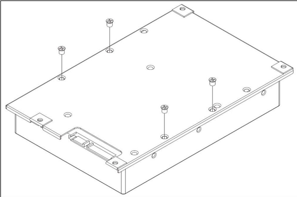
4. Mount the HDD rack back to its original position. No SATA cable required; the HDD is connected automatically.
