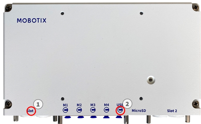
Fig. 3: CNPP compliant connection to the S74 Camera
