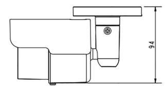
Fig. 1: 2MP Bullet Camera: All measurements in mm
