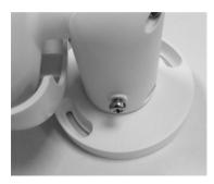
2. If the screw holes are blocked by the camera body, loosen the screw shown in the right figure but do not detach it. Then rotate the camera body to reach the screw holes.
