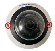
2. Place the camera at the installation location (when installing the camera to a wall, the cable entry should always be at the bottom). Mark the position of the two screw holes indicated by the red circles in the figure on the ceiling or wall (the red arrow indicates where the Ethernet cable will enter the camera).
