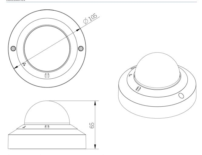
Fig. 1: 5MP Indoor Micro Dome Camera: All measurements in mm
