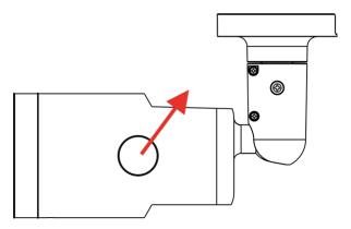
2. Open up the internal cover using a security Torx.
