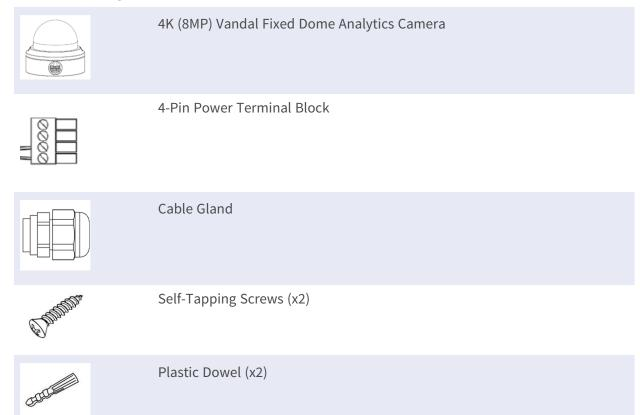
**NOTE!** The supplied self-tapping screws are for soft substances/materials such as wood. For other installation environments, such as solid or sheet rock walls, users **MUST** pre-drill and use plastic anchors before fastening the camera onto the wall.
