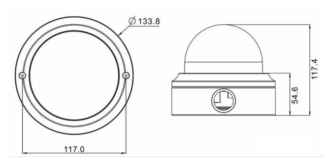
Fig. 1: 4K (8MP) Vandal Fixed Dome Analytics Camera: All measurements in mm
